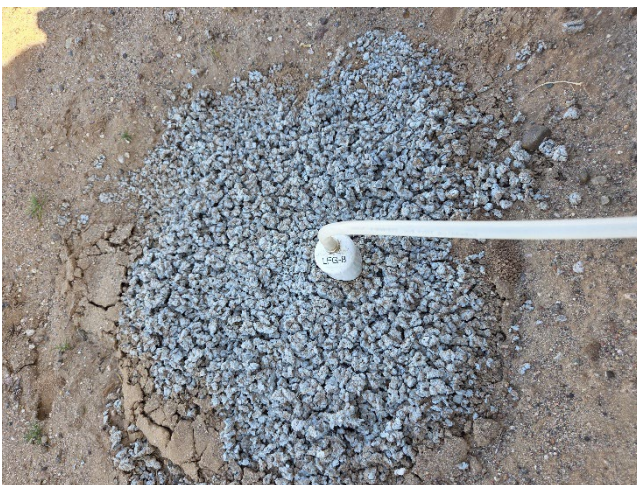
Photo 11: View of landfill gas screening at LFG-8 at the subject property.
