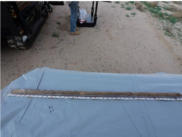
Photo 3: View of the 0- to 4-ft bgs sample from borehole B-1 at the subject property.
