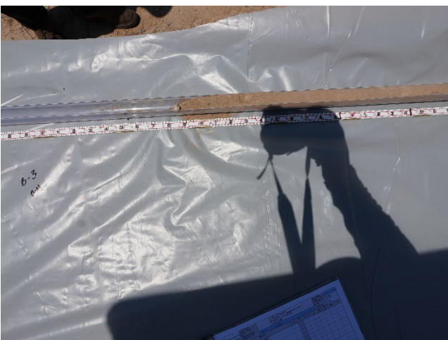
Photo 5: View of the 0- to 4-ft bgs sample from borehole B-3 at the subject property.
