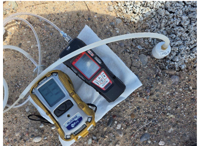
Photo 10: View of landfill gas screening at LFG-5 at the subject property.
