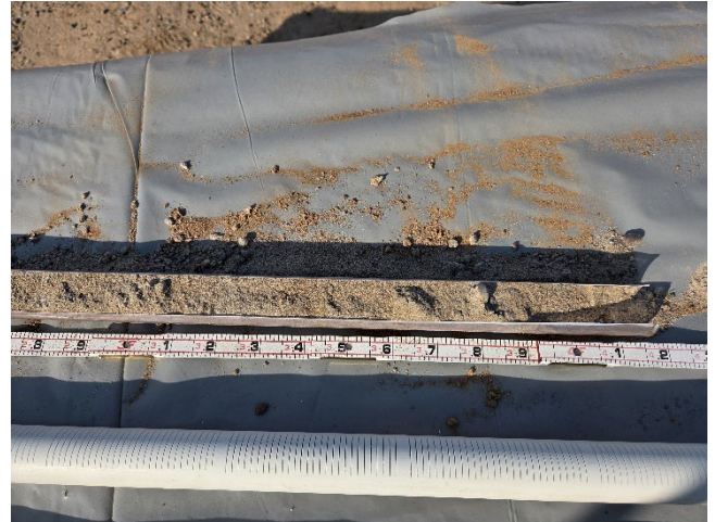
Photo 8: View of well screen next to a soil sample at the subject property.
